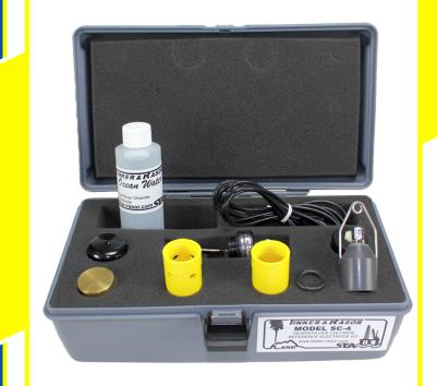
The Model SC-4 Sliver-Silver/Chloride kit come complete with everything necessary to conduct field tests both ON SHORE and OFF SHORE.
