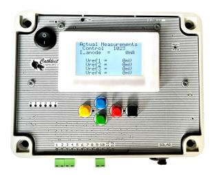
Anode Current Controller (MACC) for Cathodic Protection Systems, operating on all Sacrificial (galvanic) Anode Systems, Magnesium, Aluminium and Zinc Anodes, providing automatic potential IR-FREE control, constant current, constant potential instant "OFF" control and current pick up control for internal steel water storage reservoirs, pipelines, marine structures, fresh water dams, reservoirs with metallic structures, yachts and ships.
